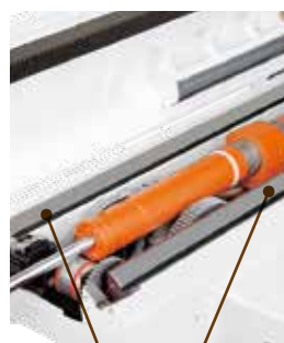
Longitudinal double "V" guideways
