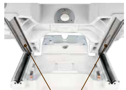
Cross feed double "V" guideways
